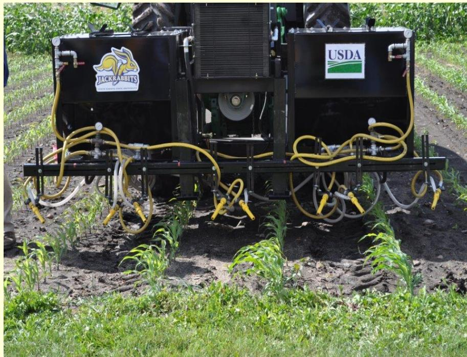
Four-row grit applicator has 8 nozzles, one for each side of four rows
